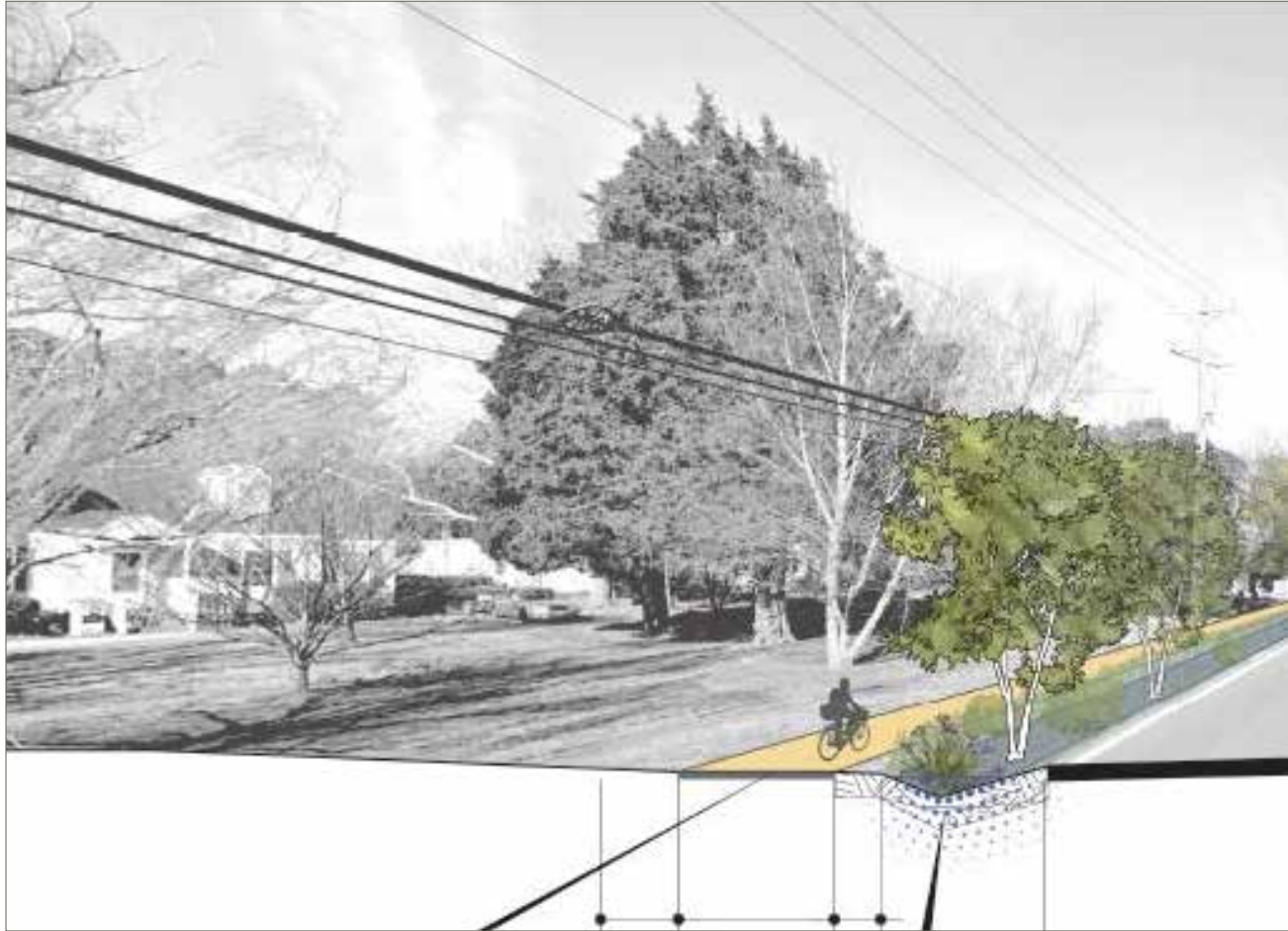
The Armistead Avenue road-raising and green infrastructure project, funded by a City of Hampton environmental impact bond, will eliminate chronic flooding on a major thoroughfare and evacuation route.
